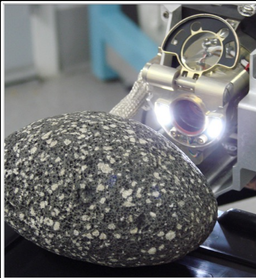
4 White Light LEDs Can control each group of 2 separately
