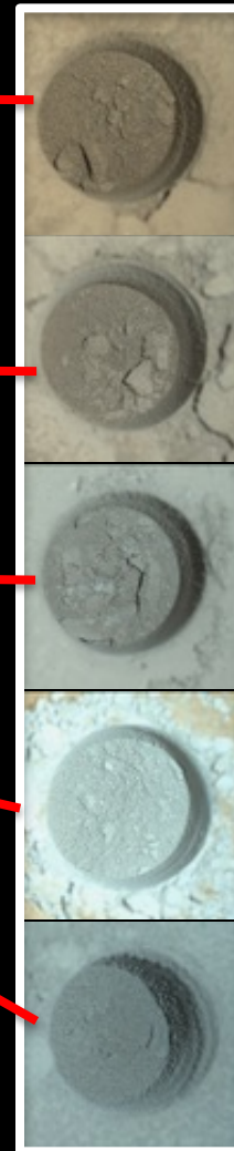
16 mm diameter drill holes
